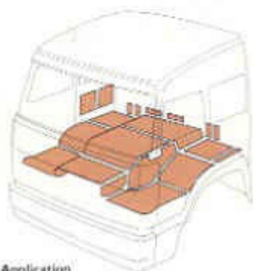
Application of fusible sound-proofing sheets.
